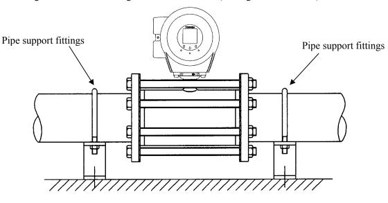
Figure 4.2 Example of Pipe Fixing Procedure
